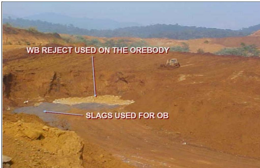
Figure 4-20: Use of Waste Material and Slag on Pit Floor (Photo PTI)
