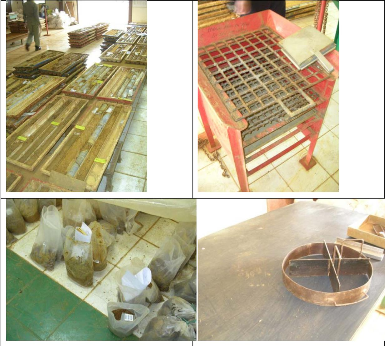
Figure 4-7: Core sample preparation
