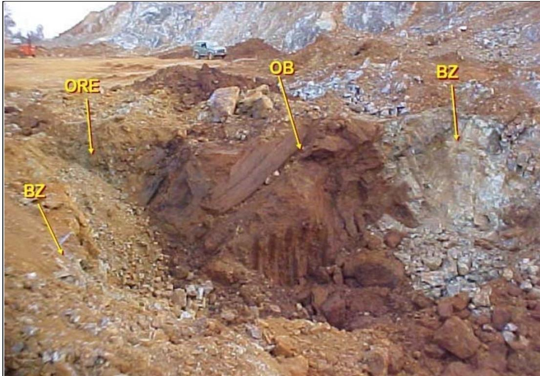
Figure 4-23: Ore Identification (Photo PTI)
